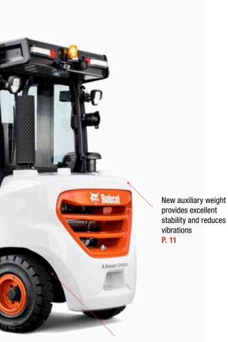
Increased steer angle reduces the steering radius, allowing for improved maneuverability P. 7
