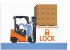
When the operator leaves the truck unattended, the hydraulic locking system prevents unintentional lowering and tilting of the mast. It safeguards the truck, the load and the operator.
