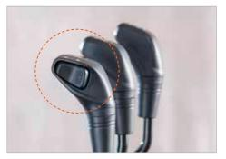
Ergonomically designed hydraulic levers with F/R switch (only B25NS Series)
