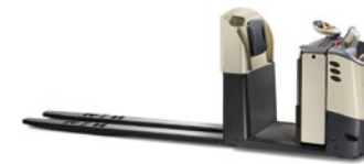
GPC 3000 Series Low-level order picker Max. truck capacity: 2,500 kg Max. lift height: 240 mm Available with: QuickPick Remote
