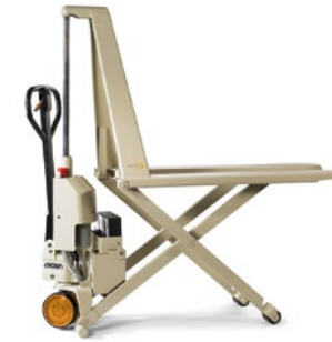
PTH 50 Series Hand pallet truck with scissor lift Max. truck capacity: 1,000 kg
