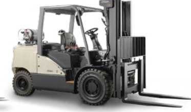
C-G 35-55 Series Four-wheel Power: Gas, LPG Max. truck capacity: 5,500 kg Max. lift height: 6,050 mm
