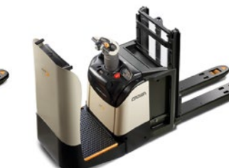
DT 3000 Series Rider double stacker with fixed platform and side entry Max. truck capacity: 2,000 kg Max. lift height: 1,670 mm
