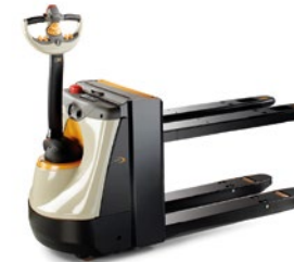
WP 3200 Series Walkie pallet truck with high lift Max. truck capacity: 2,000 kg
