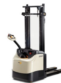
ES 4000 Series Walkie stacker with/without initial lift Max. truck capacity: 1,600 kg Max. lift height: 5,400 mm
