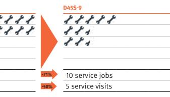
• Drive axle oil : 500hr  $\rightarrow$  2,000hr • Transmission oil :  $1,000hr \rightarrow 2,000hr$
