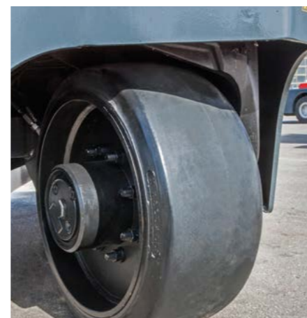
Elastic tyres with or without profile for uneven floors and outdoor operation
