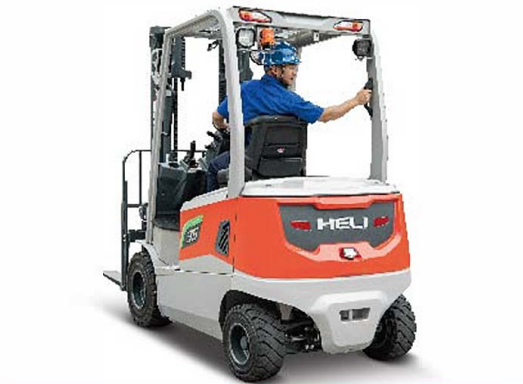
The rear handle and warning horn are designed for safer reversing operation.
