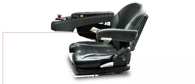
Optional grammer fully suspended seat is more comfortable to drive: The multifunctional armrest integrates fingertip switch, direction switch, steering switch, PES gear, horn button, emergency power-off switch, etc., to realize convenient operation and precise control of electromagnetic proportion.
