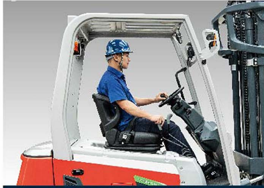
Right positioned control valve is more comfortable.
