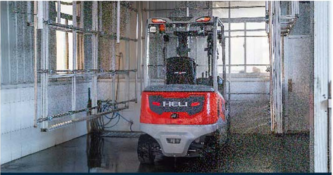
IPX4 waterproof: the vehicle is powered on to simulate a 15min short-time 5000L rainstorm test, and the vehicle can continue to run without failures.
