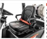
**COMFORTABLE** ALL SHIFT LONG Work through your shift in comfort with many quality-oflife features as standard: ergonomic seat, easy-to-read instrument panel, tiltable steering column, anti-slip plate, and more. P. 8-9
