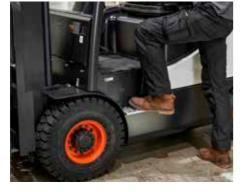
This forklift features a low step height, facilitating easy and safe operator entry and exit, complemented by an easy entry grab bar and an anti-slip step plate.
