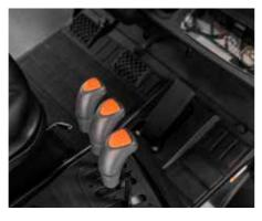
Effortlessly control with automotive-style pedals—large accelerator, inching, and air-boosted power brake. Brake with ease, even when the engine is off, thanks to the spring-actuated parking brake handle.
