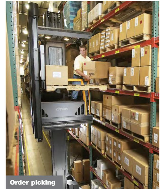
Sturdy steel side gates and a clear front rail reduce the need for operators to bend or lean when retrieving products from racks or placing them on pallets. The rails can also be used to support the weight of a product as it is transferred to the pallet.
